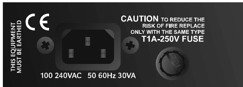
Location of mains fuse on rear panel.
