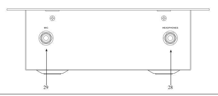
**28. HEADPHONE OUTPUT JACK -** This jack is used to connect your headphones to the mixer allowing you to monitor the cue source. Use headphones only rated at 8 ohms to 32 ohms. Most DJ headphones are rated at 16 ohm, these are highly recommended. Always be sure the CUE LEVEL VOLUME (5) is set to minimum before you put the headphones on.
