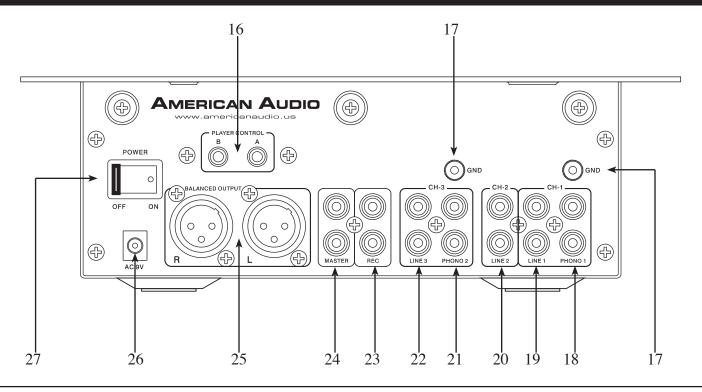
**16. PLAYER CONTROL** - These jacks are used to control the "Q-Start" function between the mixer and a compatible American Audio CD Player. Input mini plugs from CD player controller into these jacks, input CD 1 into jack A and CD 2 into jack B.
