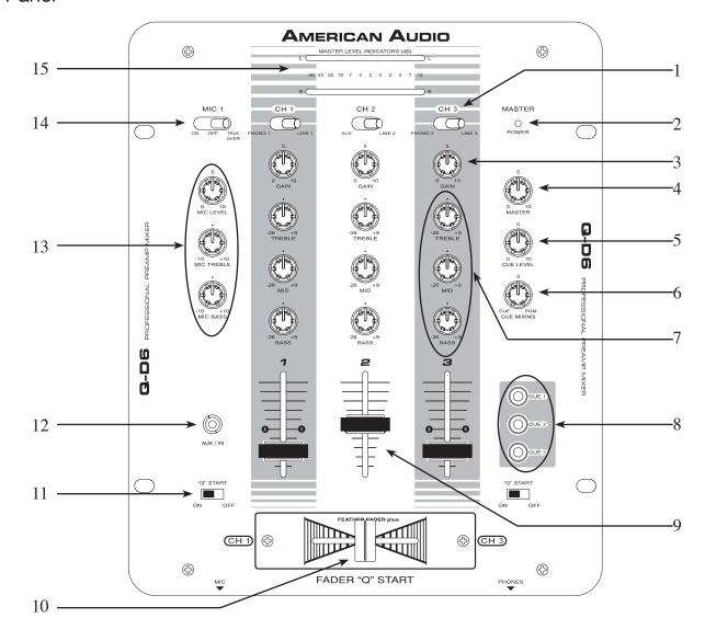
**1. SOURCE SELECTOR SWITCH -** These switches are used to select the input source assigned to each channel. Each channel may only be assigned one input source at a time. This switch must be in the "phono" position for turntable operation.
