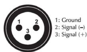
DMX-input XLR mounting-plug:
