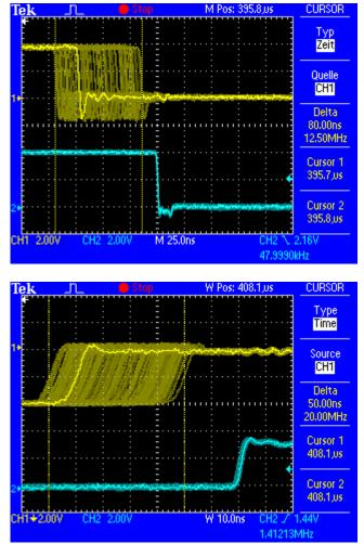
The cleaned and jitter-freed signal can be used as reference clock for any application, without any problem. The signal processed by SteadyClock is of course not only used internally, but also available at the XTC's word clock output. It is also used to clock the digital outputs MADI, ADAT and AES/EBU.
