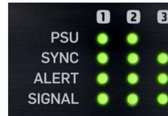
*Fig. 15.: Front panel indicators on Loudness Pilot with three SDI cards*
