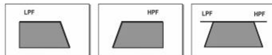
Signal segment obtained with the combination of LPF and HPF .
